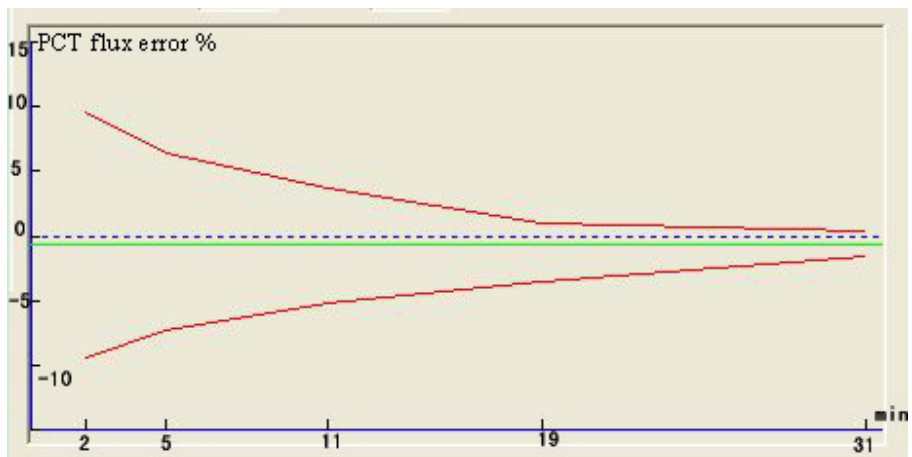
Fig. 5.2.2 Horn-shape curves when the rate is 1ml/h
